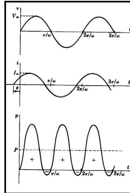
$$P = I_{\text{eff}} V_{\text{eff}} \cos \theta$$
