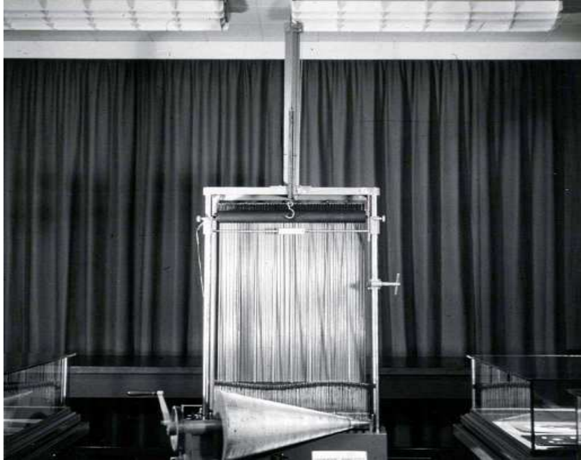
Figure 3.1.1: The harmonic analyzer built by Michelson and Stratton
