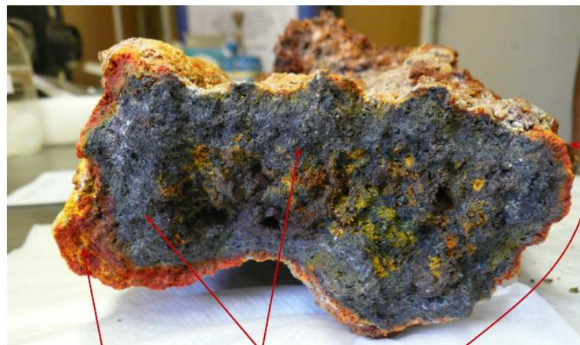
As-sulfide phase Massive sulfides & sulfates CORE Brown Fe-containing coating 29
