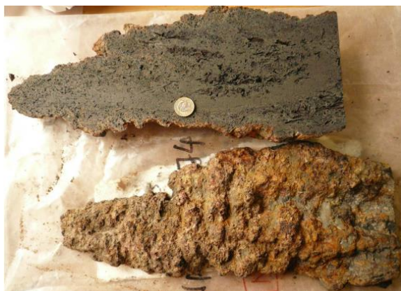
Grey bacteria mixed with brown Fe-containing coating As-sulfide phase Massive sulfides & sulfates CORE 28
