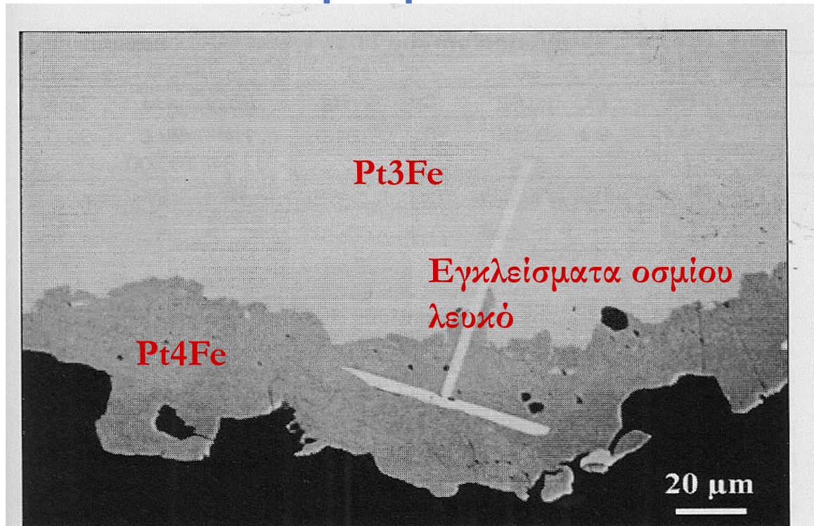
Fig. 105-1. SEM photomicrograph showing part of a magnetic Pt 3 Fe alloy nugget with a rim of tetraferroplatinum (darker) and two osmium inclusions forming the outline of a geological hammer. The later tetraferroplatinum has replaced the Pt 3 Fe alloy, but not the earlier exsolved osmium. Placer sample BM1928,246 (grain 8) from Yubdo (see Cabri et al., 1981, for details on the locality and provenance).
