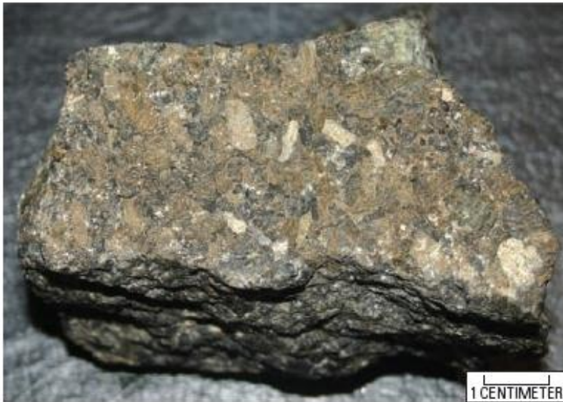
Figure 27. Typical chromite-bearing rock from the Stillwater Complex. Photograph courtesy of Bruce Lipin, U.S. Geological Survey.
