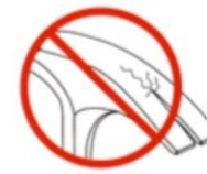
Crack in claw section
